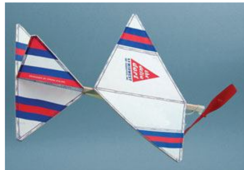
This is the Delta Dart, a.k.a. the AMA Cub. It's an easy-to-build beginner model. See vendor list for more information. The balsa wood framework is glued direct to the plan which become the model's covering after trimming around the outlines.
